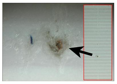
**NOTE:** This cable originates at the controller card's **11** header and terminates at the flatbed CCDM. It is where this cable passes through the steel frame of the flatbed where the damage occurs.
